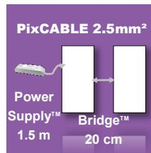
They connect one **PixBOARD™** to another (**PixCABLE BRIDGE™**) or to the transformer (**PixCABLE POWER™**).
